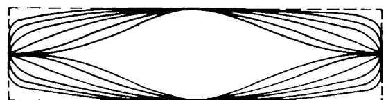
Fig. 4 Slot planform shapes for the family t(x) = [4x(1-x)]^{\sigma_n} where \sigma_n = 4, 2, 1, 1/2, 1/4, 1/8 (from pointed to blunt).
